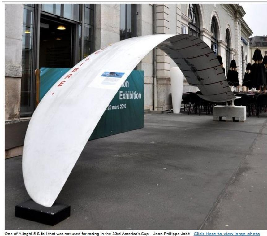
Figure 2- A huge S type daggerboard from Alinghi 5 built for the 33rd Americas Cup
