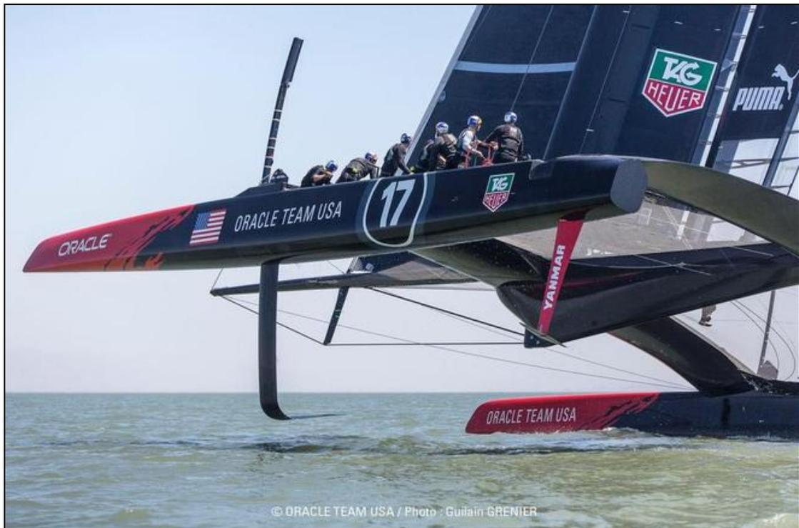
Figure 1 - Team USA Boat No2 in training with the L shaped port daggerboard clearly seen. Plus the machined aluminium prototypes rudder elevators are bolted on so modifications can be made easily. Once the design is settled carbon fibre versions are made to reduce weight.
