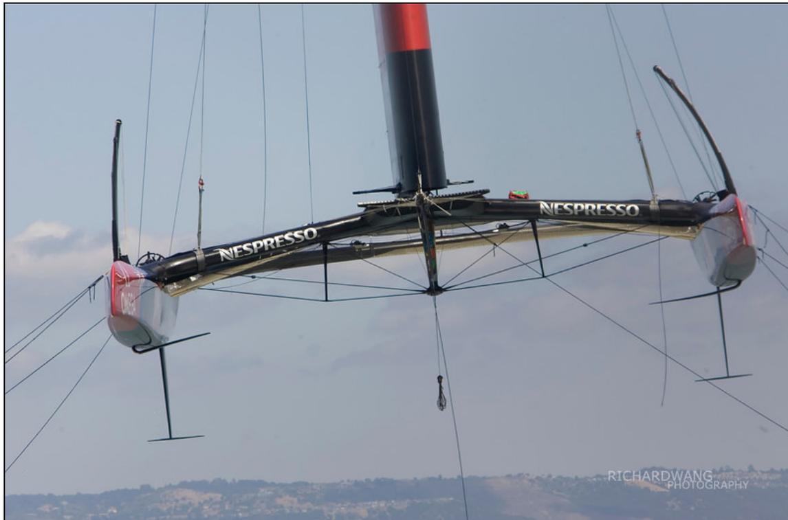
**Figure 7 - Team NZ with two slightly different foils installed. What better way to sort out differences just by sailing port and starboard courses!**
