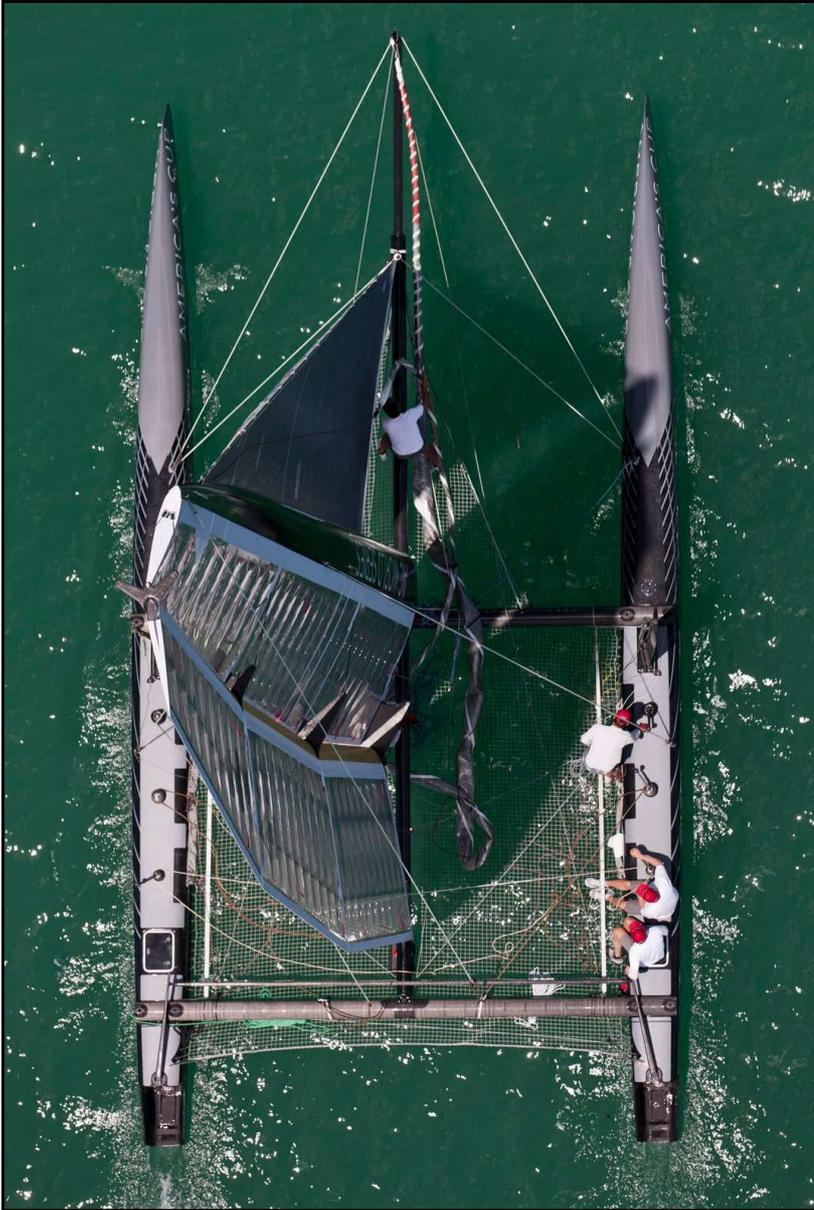
**Figure 3 – Cambered Wing but no twist**
